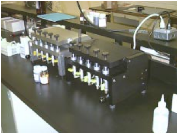
Figure 14, Multi-station RFS Sample Preparation Fixture
