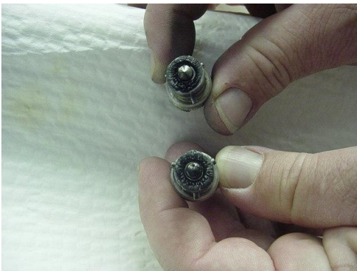
Figure 7. Defective Magnetic Chip Detectors (MCD)
