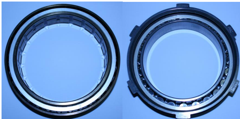
Figure 3. #4 and #5 Bearings Removed from F110-GE-100 Engine
