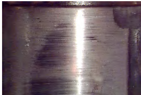
Close up of the wiped bearing
