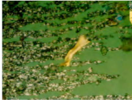
Fig.3 Photomicrograph indicating an isolated copper particle. Magnification 500X
